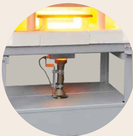
15 kW propane gas mounted under the kiln
