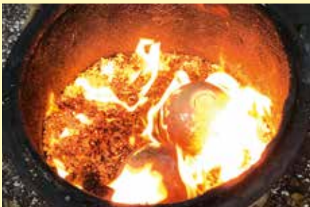
Cool down and immerse the material to be burned in leaves, straw or shavings
