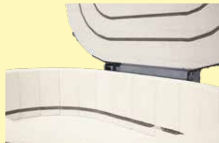
Kiln interior with circular lower side heating
